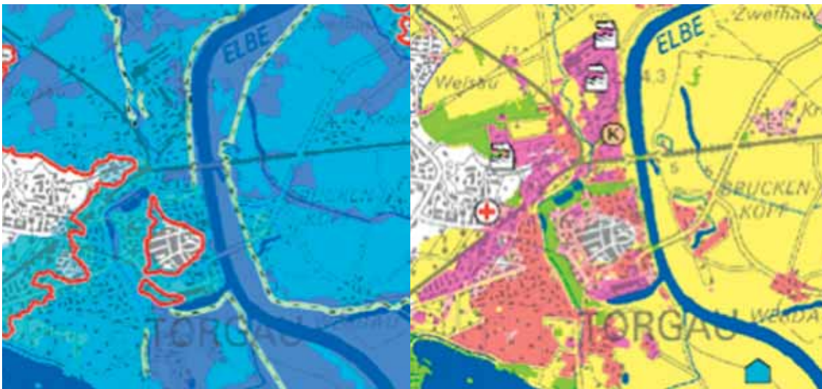
Portion of Flood Map and Damage Potential Map in the Saxon Flood Risk Atlas
