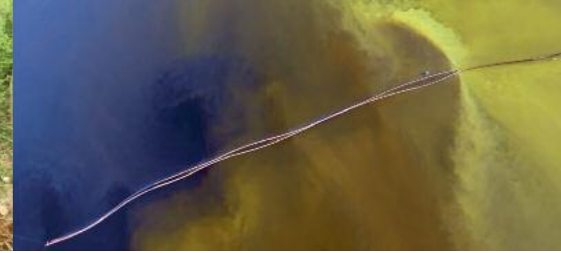
neutralisation of the post mining lake „Scheibese“, lime slurry spreading by using input cable
