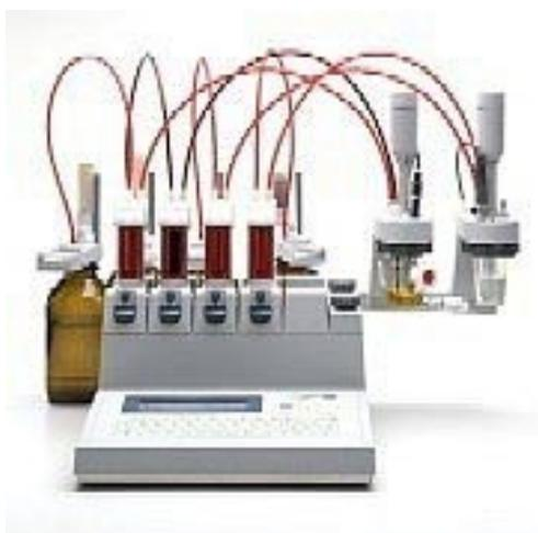
High performance titrator with greatest method and automation flexibility. The titration software is included for complete overview and control from the PC.
