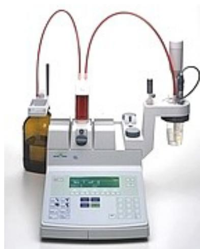
The DL53 is a routine titrator. Concentration determinations are quick, economical and highly reproducible. The system has up to 2 precision burets. Easy operation and PC connectivity are also characteristics of this titration instrument. The display can show the titration curve online. The titration software is included for complete overview and control from the PC.
