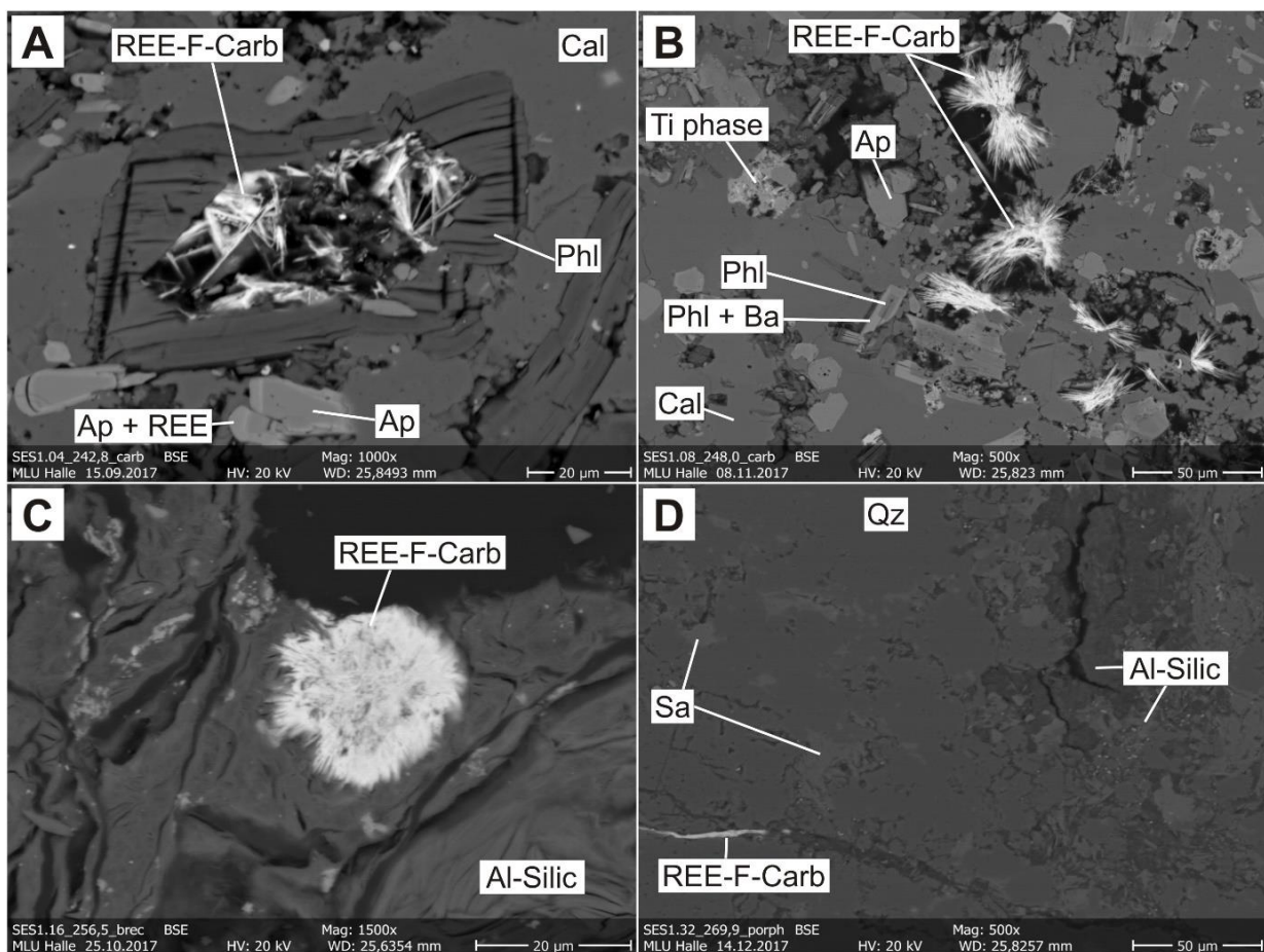
Figure 43: Typical REE-fluorocarbonate occurrences (SEM-BSE); A: Small needle-shaped crystals in cavity in alvikite section; B: Larger aggregates from the alvikite sample SES1.08; C: Typical aggregate from a breccia section with grey matrix; D: REE-fluorocarbonate vein in the porphyry section. The occurrence of the vein shows, that there was a small impregnation of the wall rock by the intrusion or hydrothermal fluids.
