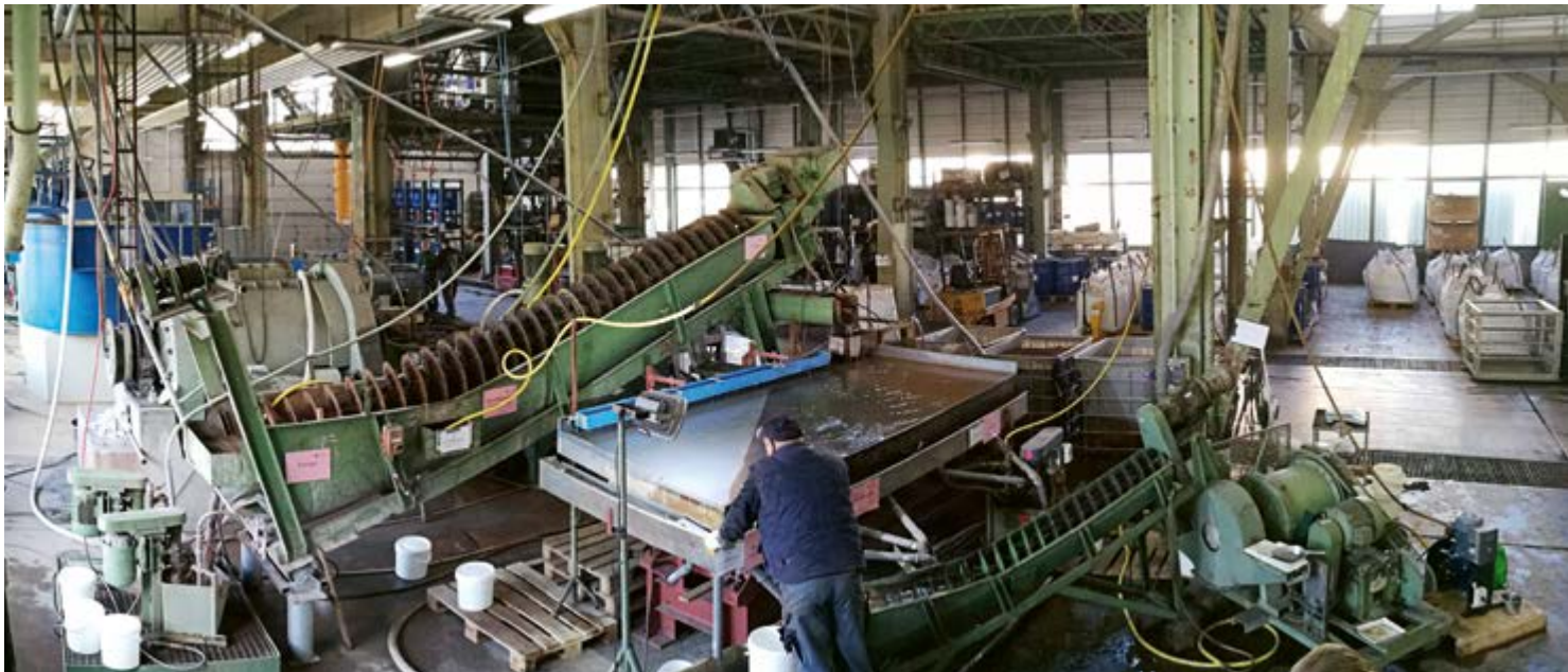
Illustration 32: Pilot plant for the extraction of sulphides, cassiterite and magnetite from a bulk sample (Source: UVR-FIA GmbH 2018)
